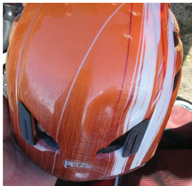
DAMAGED PETZL METEOR FOLLOWING A GROUND FALL OF ~10M ON HEAVEN CRACK, STANAGE EDGE.
